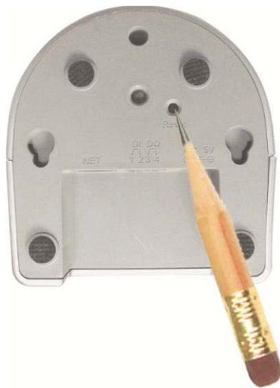
Figure 3-31: Stick on the reset button to set to the factory default
